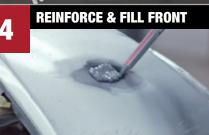
Remove tape from front. Fill front with *Dual-Mix* Multi-Plastic Repair Material or *Dual-Mix* Problem Plastic Repair Material. Spread material firmly and build up higher than panel to allow for sanding.
