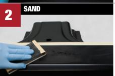
Sand primer with P180 grit. Sand bare metal with P80 grit. Blow off and tack clean. Re-clean with SEM Solve or XXX Universal Surface Cleaner. Wipe clean in one direction with clean, lint-free cloth.
