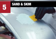
Sand with P80 grit. Finish with P180 grit. If needed, use a skim coat of **BUMPER BITE™ Flexible Glaze**, then sand with P180 − P320 grit.
